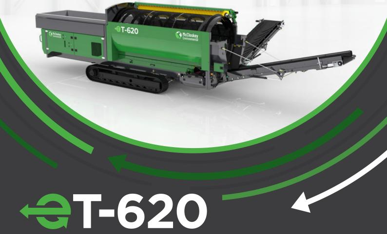
The ET-620 is a tracked trommel designed specifically to meet the needs of the European and ROW market. The ET-620 has been designed to meet the needs of plants dealing in wood waste, compost, Light C&D waste and general MSW.
